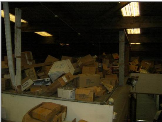
Figure 1 - Excessive internal storage of combustibles – increased building fire load.
