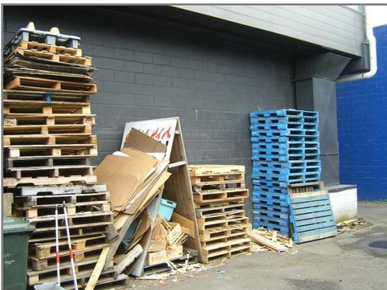
Figure 3 – Combustibles at rear of a commercial building – a serious arson risk.
